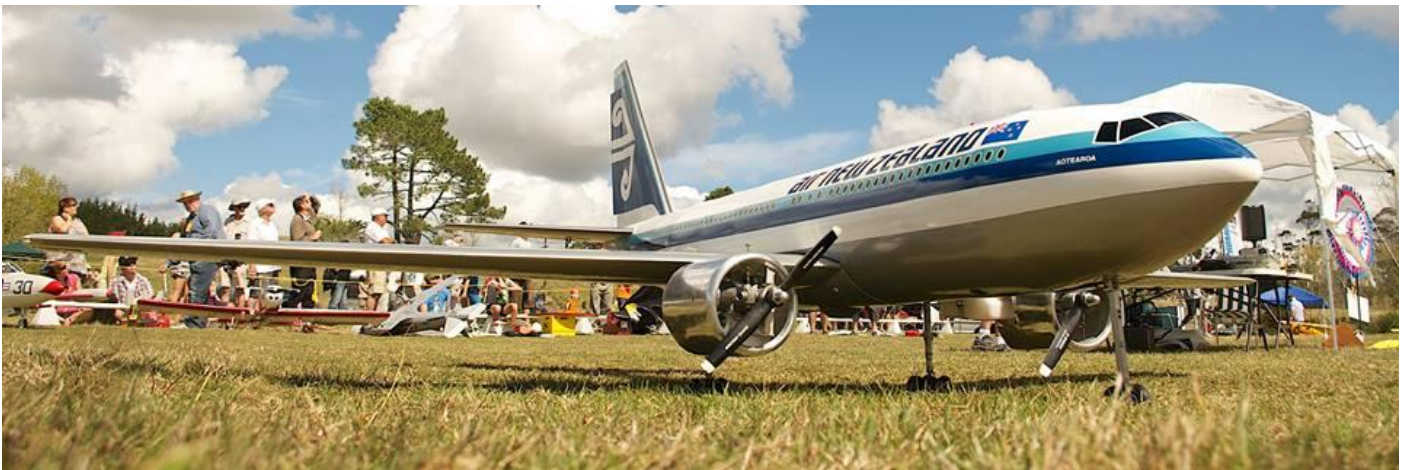
The Boeing 767, twin OS 108's and 16kg servos except the ones on the throttle which have been upgraded with traxxas water-proof car steering servos. Now it's just waiting for flight
